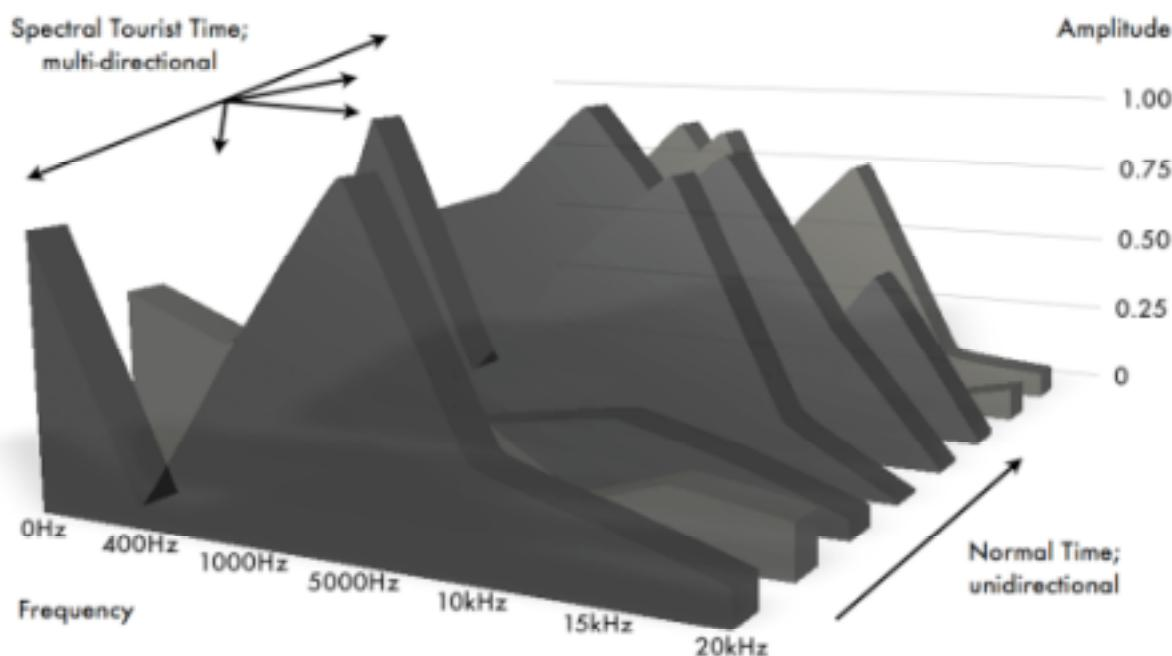
*Figure 1. Sheets of spectral data are lined up in normal time. The Spectral Tourist can travel forwards and backwards and morph from sheet to sheet in multiple directions controlled by the joystick. It is easy to get lost and to take a wrong turn while navigating this space.*
