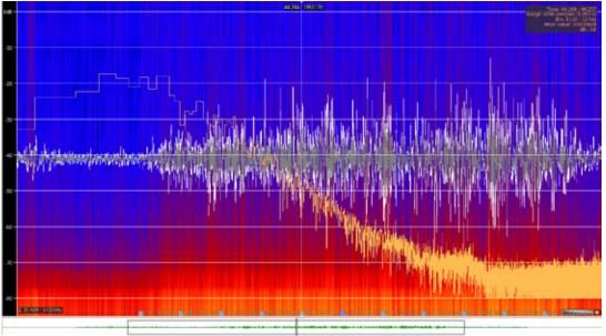
MMG of a sustained contraction: spectrogram (in the background); waveform (white in the foreground); and logarithmic spectrum (yellow outline).
